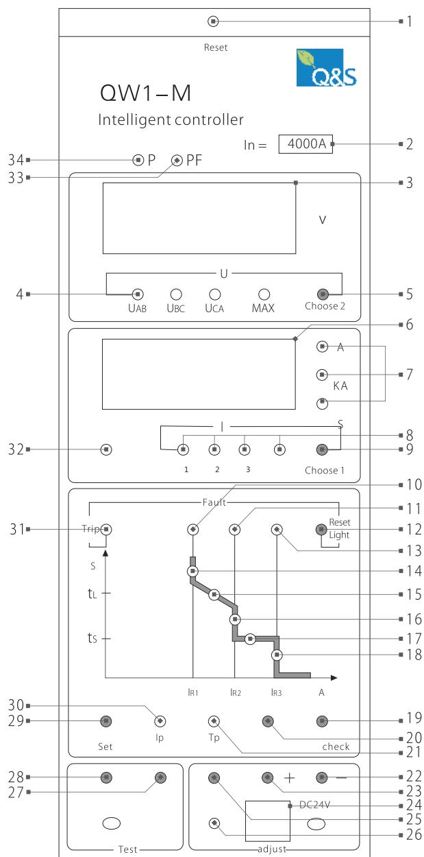
Figure : QW1-M-type control panel introduction
